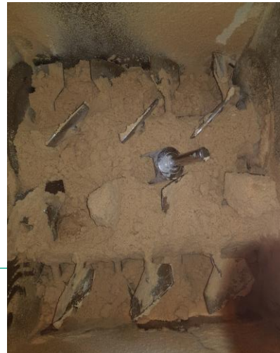
Twin-shaft mixer with 24 paddles – difficult cleaning
