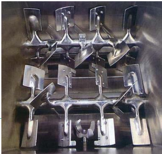
Twin-shaft mixer with 24 paddles – difficult cleaning
